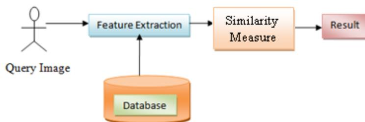
Figure 1. Block Diagram of CBIR
